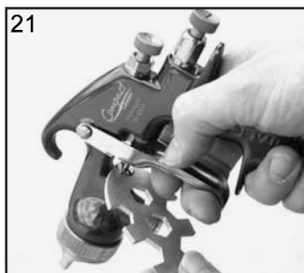
21. Adjust Needle Packing (4) with Spanner sufficient to seal but to allow free movement of needle. Lubricate with gun oil.
