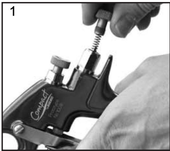
1. Remove Adjusting Knob (7), Spring (8), and Needle (9).
