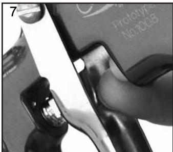
7. Push out the Front Air Valve Seal with a finger.
