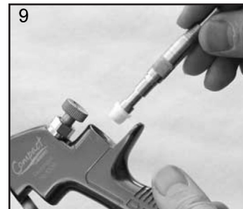
9. Fit New Front Seal to Service Tool.
