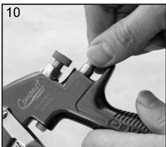
10. Fit new Seal to gunbody and press firmly to ensure Seal is engaged.
