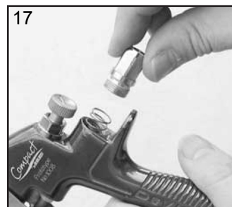
17. Replace Valve Spring and screw in Housing (10).
