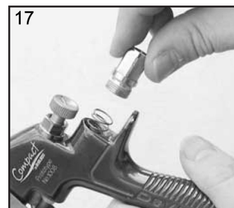
17. Replace Valve Spring and attach Housing (10).
