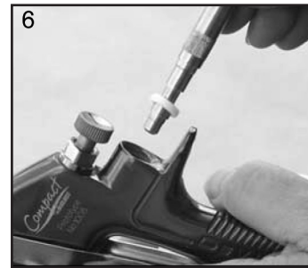
6. Remove Valve Seat.
