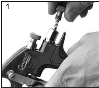
1. Remove Adjusting Knob (7), Spring (8), and Needle (9).
