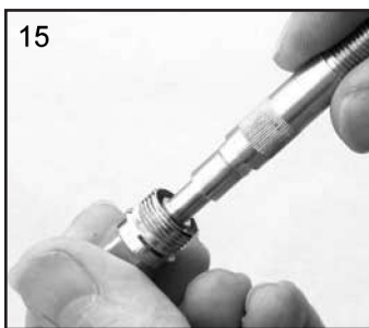
15. Fit Seal to Housing (10).
