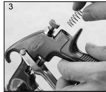
3. Remove Housing (10) and Air Valve Spring.
