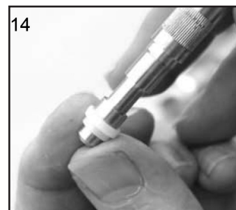
14. Fit new Seal to Service Tool.
