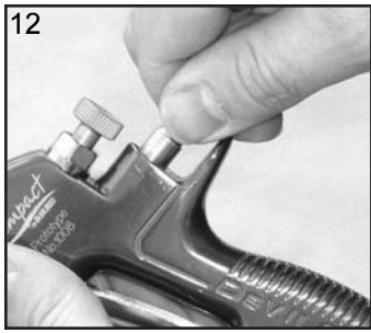
12. Fit Valve Seat to Gunbody.
