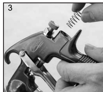
3. Remove Housing (10) and Air Valve Spring.
