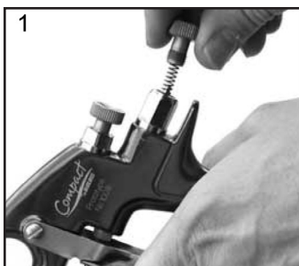
1. Remove Adjusting Knob (7), Spring (8), and Needle (9).
