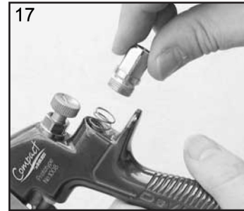
17. Replace Valve Spring and screw in Housing (10).
