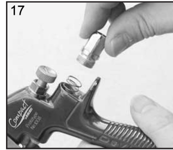
17. Replace Valve Spring and screw in Housing (10).
