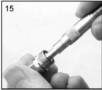
15. Fit Seal to Housing (10).
