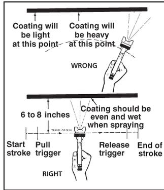
For best results, use 3 to 6 psi fluid pressure. Higher than 6 psi fluid pressure may be required for heavy-bodied materials. Low fluid pressures will produce a narrower than normal spray pattern. Generally use up to 20 psi air at **GUN INLET**. Unusually heavy, difficult to atomize fluids may require up to 26 psi air at gun inlet.
