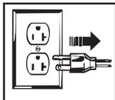
**DE-ENERGIZE, DISCONNECT AND LOCK OUT ALL POWER SOURCES DURING MAINTENANCE**
